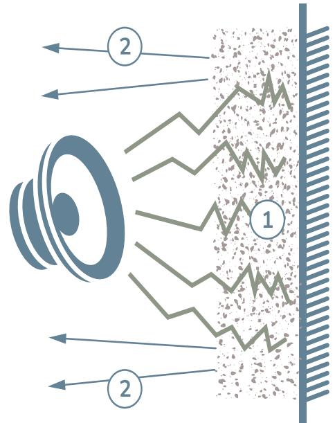
① Noise and sound is absorbed by the acoustic material
