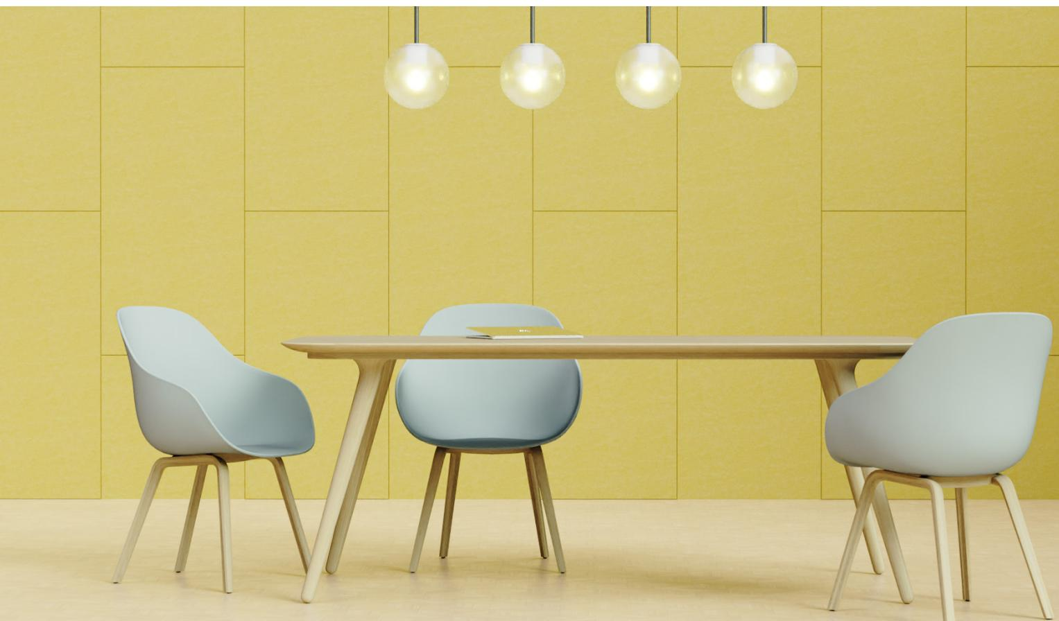
In response to the challenges of traditional acoustic dimensioning, felt and felt panels, particularly those manufactured from recycled polyethylene terephthalate (PET), have emerged as an increasingly popular and effective solution for interior acoustics. These products offer a unique combination of sophisticated aesthetics and high-quality sound insulation properties, effectively reducing unwanted noise and reverberation while enhancing interior design.
